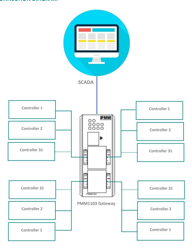
**Note:** the connection between PMM1103 gateway and the controllers can be: Modbus RTU (2 wires), or Wi-Fi or LoRa.
